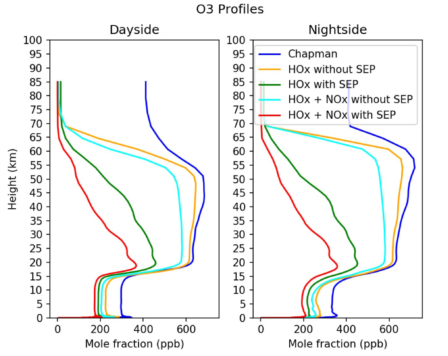
Figure 1: The average vertical dayside and nightside profile of ozone concentration.
